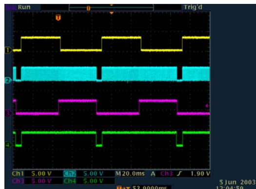
Free Run Synchronize (FRS) STROBE: Yellow = trigger, Blue = LVAL, Red = STROBE , Green = FVAL CCD:4020 Exposure = 0x0400 lines
