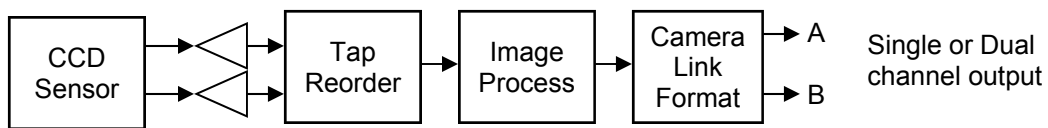
Pixel Sample to Camera Link data path
