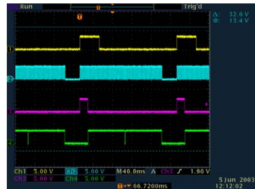
Trigger Double Exposure (TDE) STROBE: Yellow = trigger, Blue = LVAL, Red = STROBE , Green = FVAL CCD:4020 TPD = 0x1000
