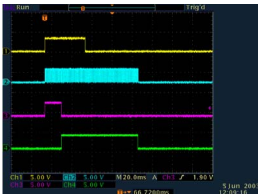
Trigger Programmed Exposure (TPE) STROBE: Yellow = trigger, Blue = LVAL, Red = STROBE , Green = FVAL CCD:4020 TPD = 0x1000
